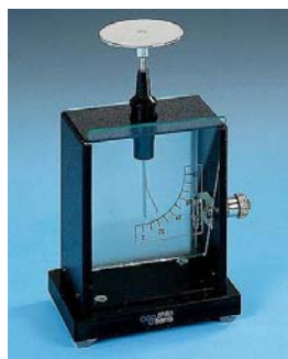
a) Aluminum leaf electroscope
