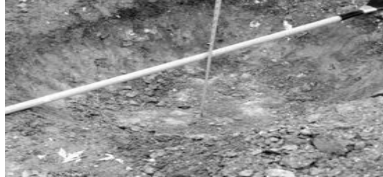
Jan. 4.3 oo muujinaya qudu bucabirka god ka Si toos ah, si gudub ah u cabbir godka, adigoo adeegsanaya mitir
