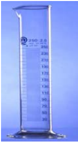
Fig 1.5 A measuring graduated cylinder
