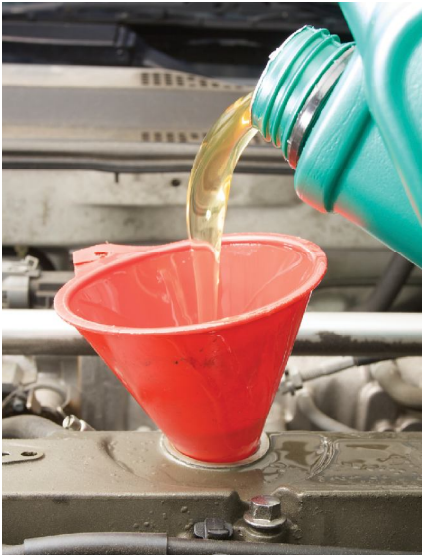
Figure 3.72 Without oil vehicle engines would heat up too much and possibly seize up entirely.
