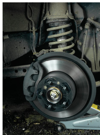
Figure 3.22 The springs used in car suspension systems need to have a high spring constant.
