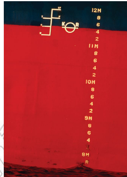
Figure 6.56 The Plimsoll line on a ship
