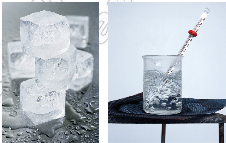
Figure 7.6 The freezing point and boiling point of water were the two fixed points used on the Celsius scale.
