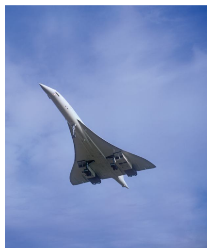
Figure 7.18 When Concorde flew at over twice the speed of sound, it got so hot that it increased its 61.6 m length by about 30 cm.
