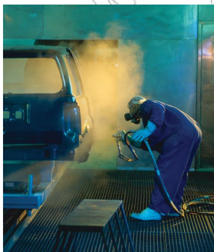
Figure 2.17 An electrostatic spray gun in use.
