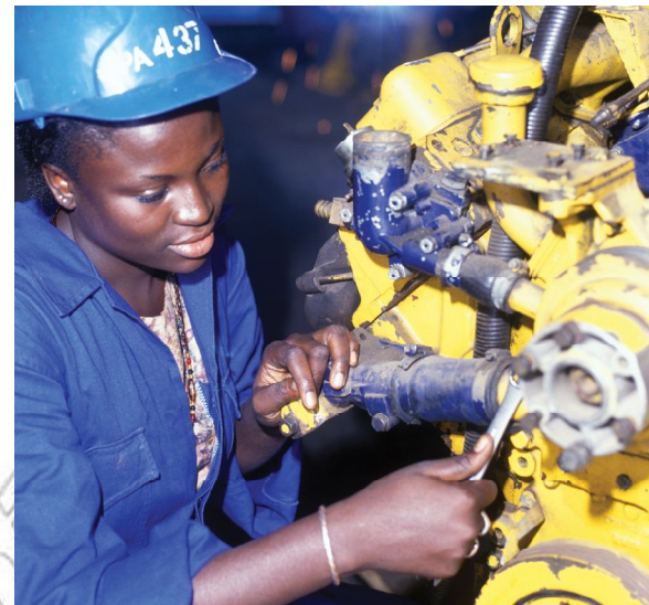
Figure 6.3 A mechanic uses torque to tighten up and undo nuts.
