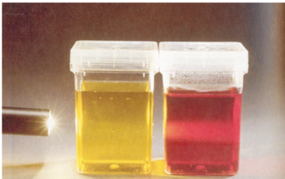
Figure 1.2 The light beam is not visible as it passes through a true solution (left), but it is clearly visible as it passes through colloidal mixture (right).
