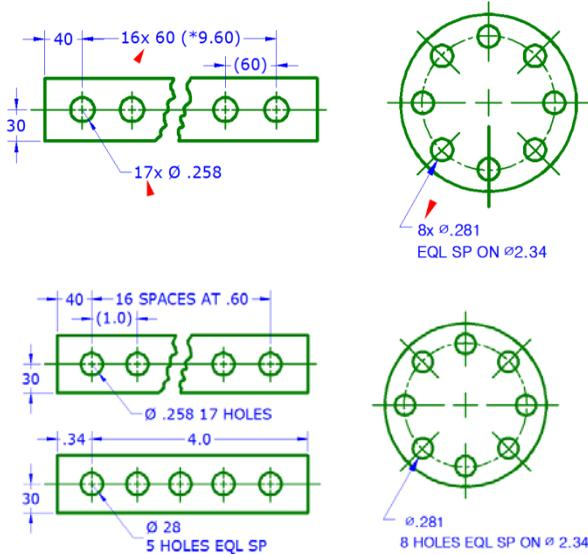
**Fig. 4.19 Dimensioning of repeated features**
