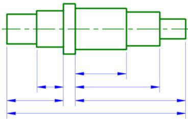
**Fig. 4.11 Combined dimensioning.**
