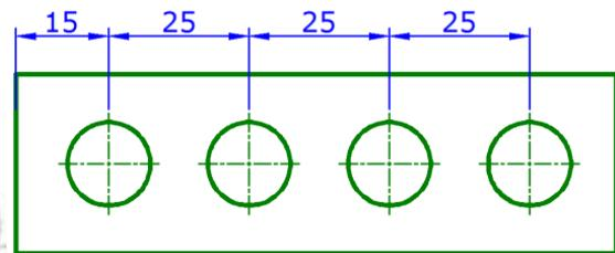
**Fig 4.9 Chain dimensioning**
